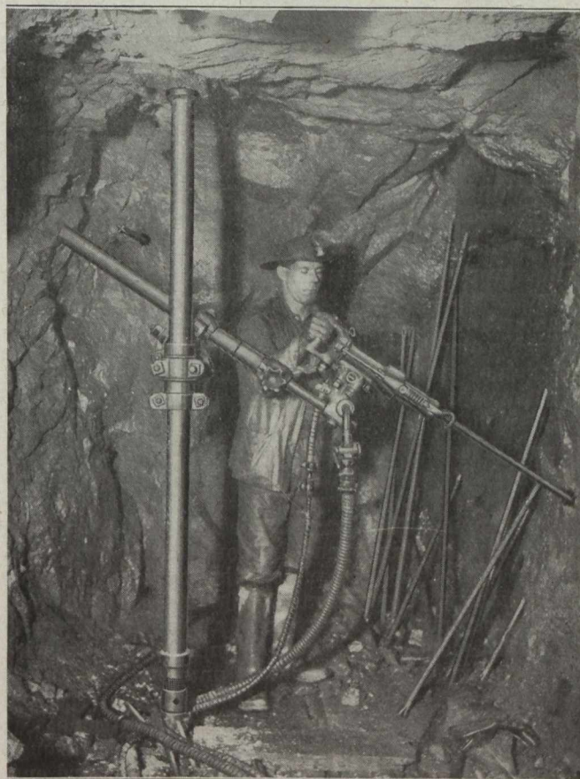
Sullivan "DP-33" Water Tube Rotator in use on pneumatic feed and "U-20" Column for drifting
