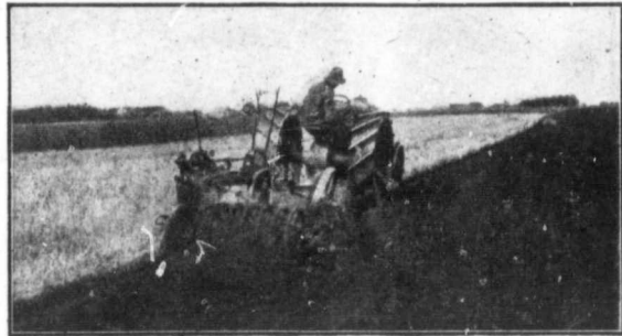
Sawyer-Massey 11-22 four cylinder Kerosene Burning Tractor doing the heavy work on the farm.
