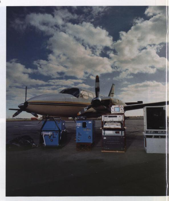
GASPILS — Another MONITEQ airborne remote sensor, GASPILS, measures hydrocarbons and other gases with absorption features in the thermal infrared (IR). Applications include gas pipeline and oil spill monitoring, chemical warfare agent detection, chemical leakage and perimeter monitoring.
