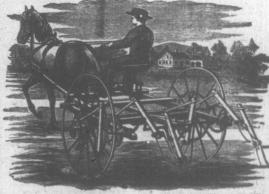
Experience has demonstrated the fact that a good HAY TEDDER that will thoroughly spread long, heavy grass, taking it up from the bottom, tossing it gently into the air, and leaving it upon the ground in a light, fleecy condition, enables the farmer to take advantage of fair weather and at least twice the quantity of hay can be segured, in better condition, than when allowed to remain in the swath.
