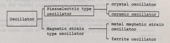
Ceramic oscillators which are usually called piezoelectric ceramics, have broad application area as follows:
