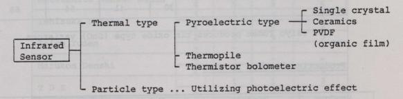
Although the particle type is superior in its physical properties, in response speed and in sensitivity, they are not suited for consumer products, due to high price and the cooling system using liquid nitrogen.
