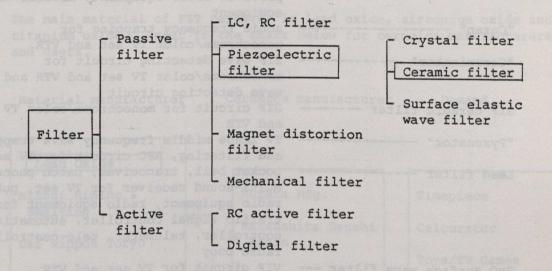
Of these, piezoelectric ceramic filters are classified by use for low frequencies or for high frequencies with major applications for TV and FM/AM radio sets.
