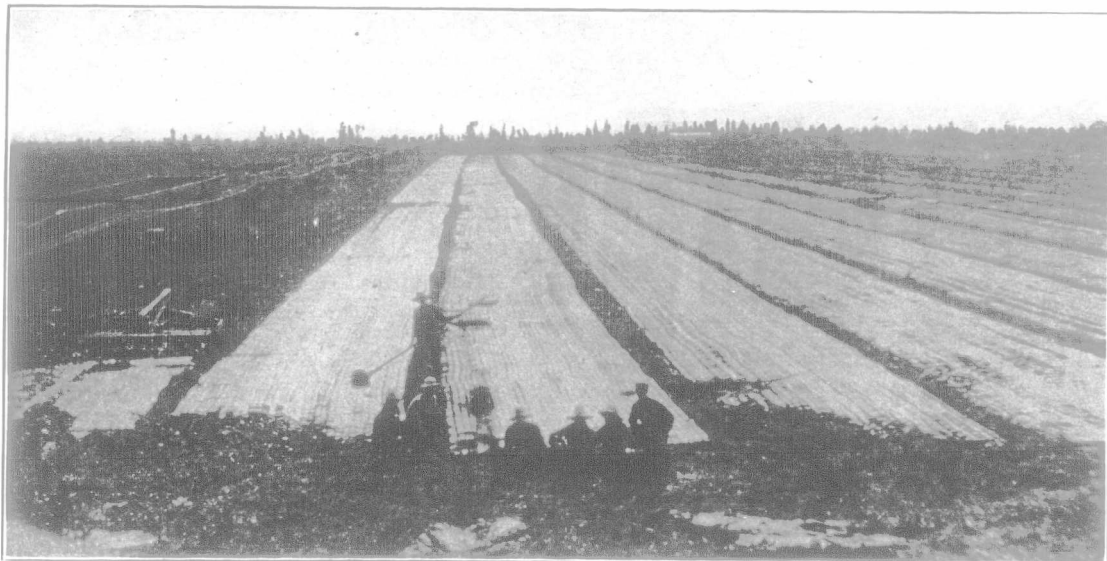
Peat laid out for drying at plant of SHUTTLEWORTH & MOORE, Alfred, Ont.
