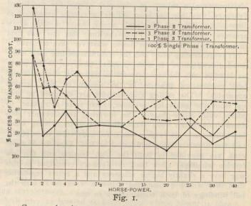
Curves showing excess of first cost of transformers for multiphase motors as compared with single phase. (These curves are based on price list of one of the large companies).
