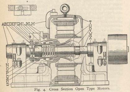
A-Pillow block cap. B-Oil cover. C-Rocker arm. D-Spring nut key. E-Spring nut. F-Adjustment stub. G-Brush holder spring. H-Carbon brush. I-Spring barrel. J-Brush holder. K-Short circuiting ring. L-Commutator. M-Terminal cable. N-Pillow block. O-Oil cock. P-Rocker arm tube. Q-Spring barrel ring. R-Governor spring. S-Field clamp. T-Dowel pin. U-Governor weight pin. V-Governor weight. W-Shaft. X-Strap bolt.
