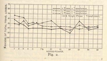
Curves showing excess of transformer losses for multiphase motors as compared with single phase.
