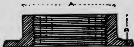
DETAILS FOR TAPPED BOSS FOR VENT FITTINGS
