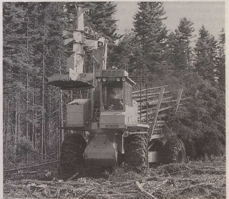
The Koehring K2FF feller-forwarder is capable of cutting trees up to 50 centimetres in diameter.
