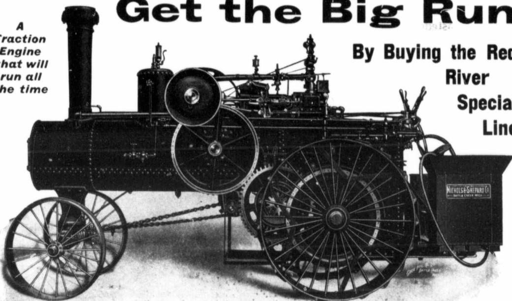
**NICHOLS-SHEPARD DOUBLE CYLINDER STEAM TRACTION ENGINE.** Built in 4 sizes—16-50 H.P., 30-70 H.P., 35-85 H.P., 30-98 H.P. Adapted to Coal or Wood. 16-50 H.P. not a Straw Burner.
