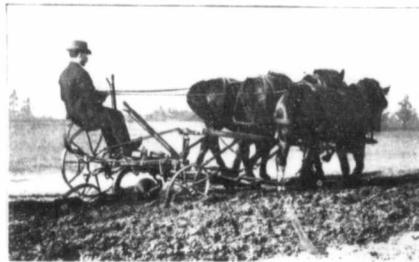
Oliver sulky and gang plows are built with the same care and thoroughness as the tractor gangs, and also have many distinctive features. The centre hitch, an exclusive Oliver feature, equalizes the pull on the horses, and enables them to walk four abreast, all walking on unplowed ground.
