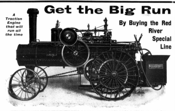
NICHOLS-SHEPARD DOUBLE CYLINDER STEAM TRACTION ENGINE. Built in 4 sizes—16-50 H.P., 20-70 H.P. 25-85 H.P., 30-98 H.P. Adapted to Coal or Wood.
