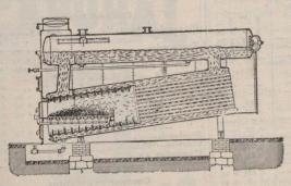
. An externally fired boiler wastes fuel because of the radiation of heat from the outside of the brickwork and the leakage of cold air above the fire, which causes a double loss by heating the excess of air and by producing imperfect combustion.
