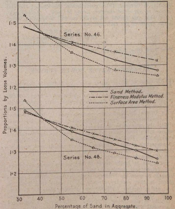
FIG. 8.—RELATION BETWEEN THREE METHODS FOR DERIVING PROPORTIONS TO YIELD CONCRETE OF EQUIVALENT STRENGTH, "FINENESS MODULUS," "SURFACE AREA," AND THE "SAND" METHODS
