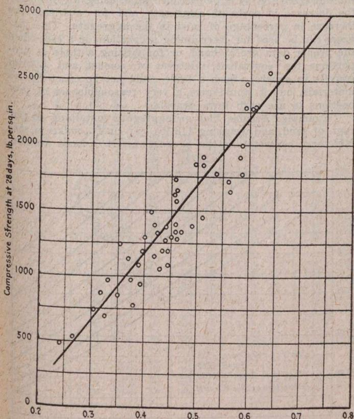
FIG. 1.—RELATION BETWEEN COMPRESSIVE STRENGTH OF CONCRETE AND THE RATIO  $c/(1-d)$
