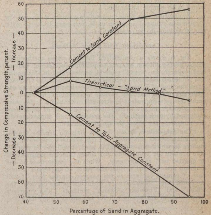
FIG. 7.—VARIATION IN STRENGTH OF GRAVEL CONCRETE, WHEN PROPORTIONED BY FOLLOWING THREE METHODS:—
