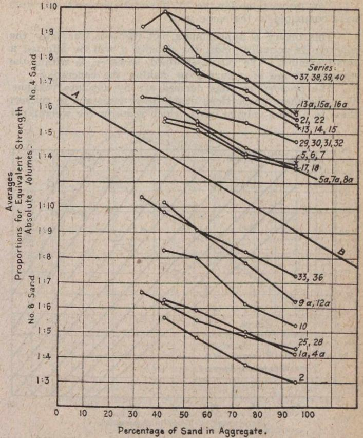
FIG. 2.—RELATION BETWEEN PERCENTAGE OF SAND IN GRAVEL, AND THEORETICAL PROPORTIONS BY ABSOLUTE VOLUME, NECESSARY TO YIELD CONCRETE EQUIVALENT TO A GIVEN BASE MIXTURE
