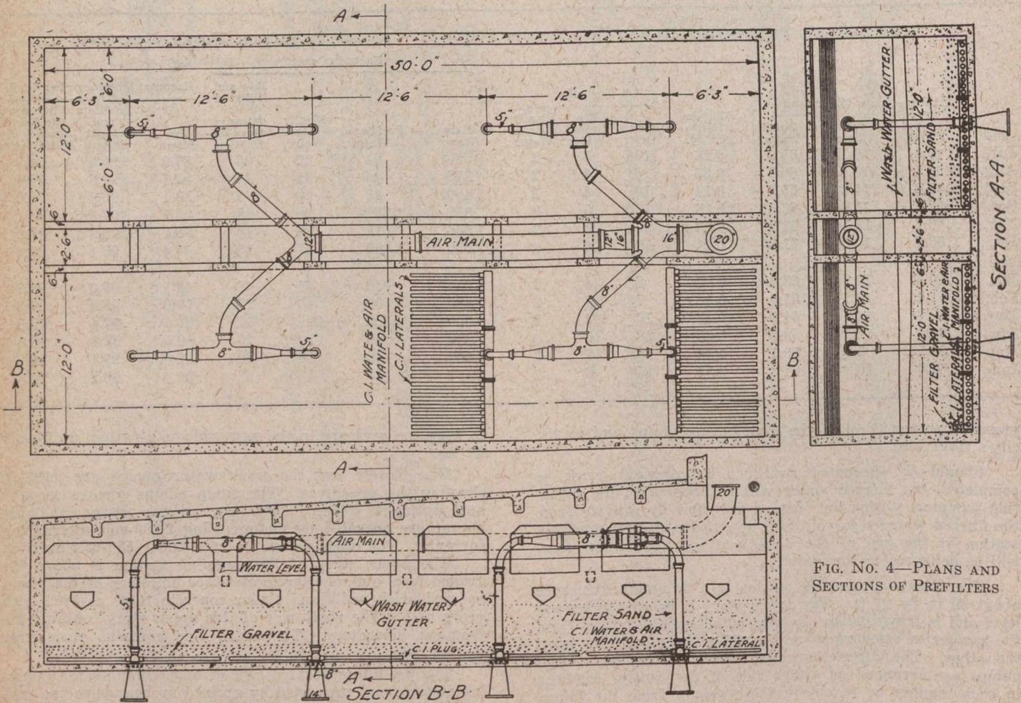
FIG. NO. 4—PLANS AND SECTIONS OF PREFILTERS
