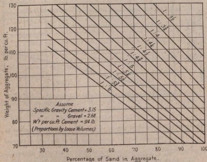
FIG. 5—DIAGRAM FOR USE IN PROPORTIONING PIT-RUN GRAVEL FOR CLASS II. CONCRETE
