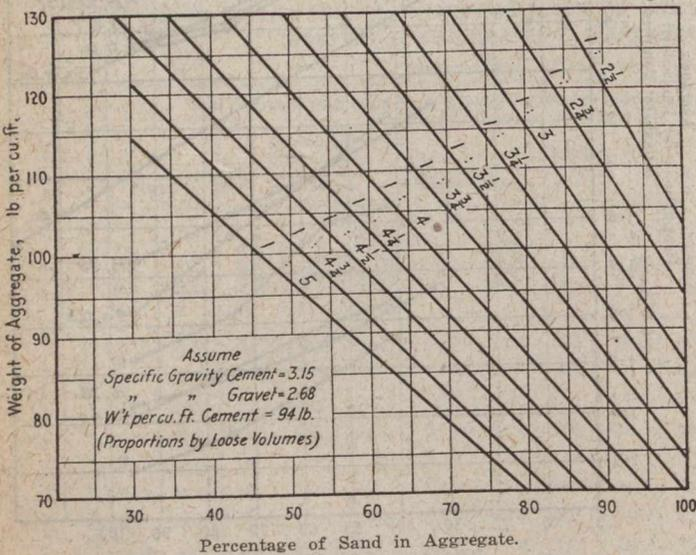
FIG. 4—DIAGRAM FOR USE IN PROPORTIONING PIT-RUN GRAVEL FOR CLASS I. CONCRETE
