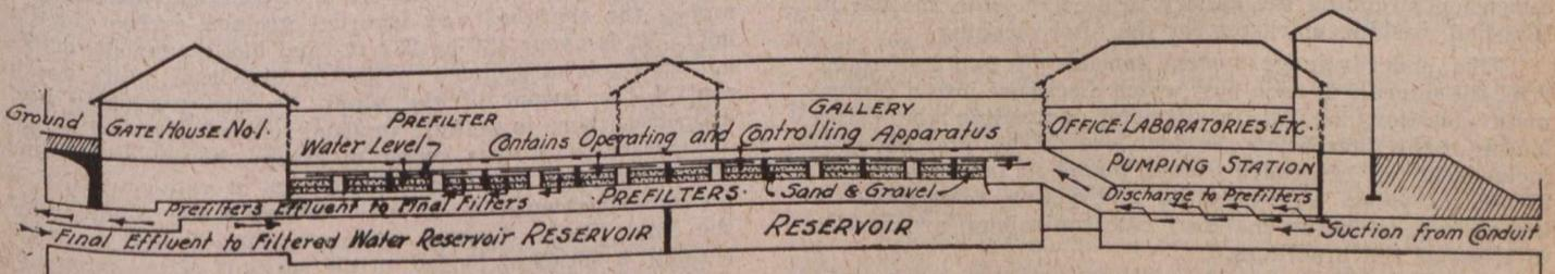
FIG. No. 3—SECTION THROUGH FILTRATION PUMPING STATION AND PREFILTERS
