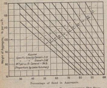
FIG. 4—DIAGRAM FOR USE IN PROPORTIONING PIT-RUN GRAVEL FOR CLASS I. CONCRETE
