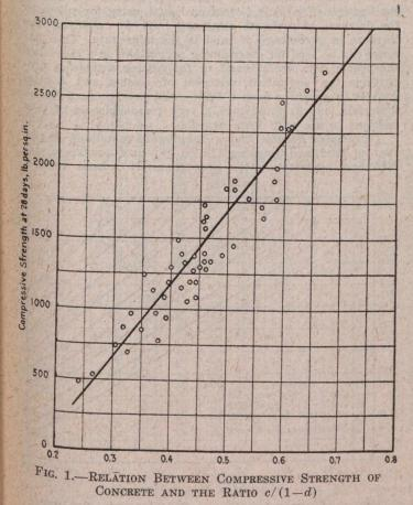
e = Absolute Volume of Cement and (1-d) = Volume of Air and Water Voids in a Unit Volume.
