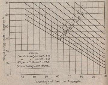
FIG. 6—DIAGRAM FOR USE IN PROPORTIONING PIT-RUN GRAVEL FOR CLASS III. CONCRETE
