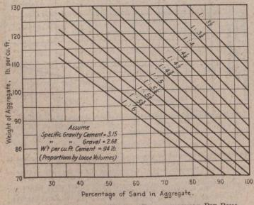
FIG. 5-DIAGRAM FOR USE IN PROPORTIONING PIT-RUN GRAVEL FOR CLASS II. CONCRETE
