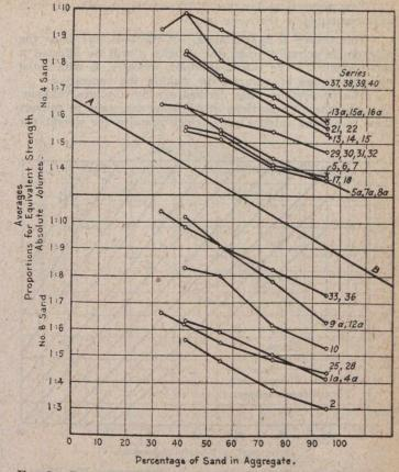
FIG. 2.—RELATION BETWEEN PERCENTAGE OF SAND IN GRAVEL, AND THEORETICAL PROPORTIONS BY ABSOLUTE VOLUME, NECESSARY TO YIELD CONCRETE EQUIVALENT TO A GIVEN BASE MIXTURE
