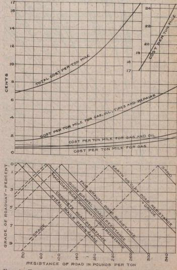
FIG. 1—TRANSPORTATION COSTS FOR MOTOR VEHICLES FOR VARIOUS GRADES AND SURFACES
