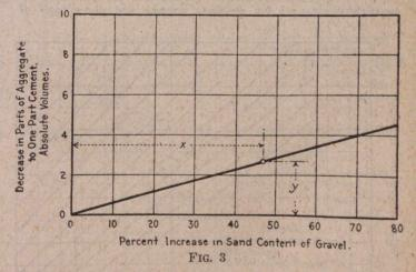
To determine the amount of cement to use with a given pit-run gravel to yield a concrete equivalent to a given mixture of sand and gravel: Reduce the proportion of the standard mix to the basis of absolute 1. volume
