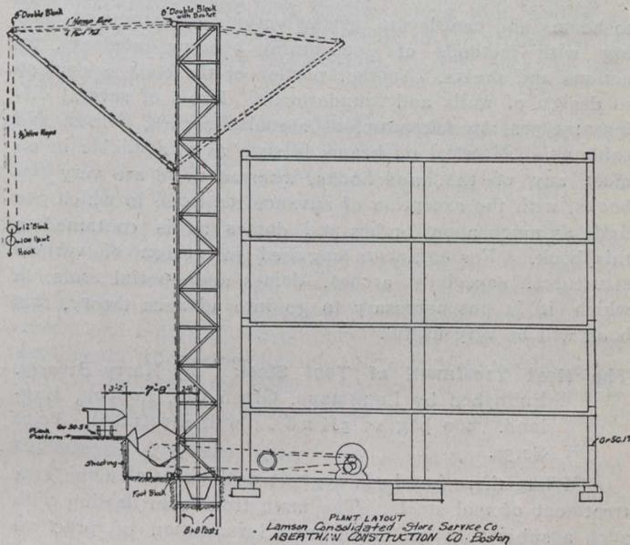
After examining the ground it was decided to place the mixer and hoisting tower at the north side of the building and to omit the building of one bay at the west end of the ground floor, so as to allow industrial cars with the coarse aggregate to be pushed through at the proper grade. Quick unloading chutes, extending from the side of the standard gauge cars were used, the material being dumped into a square-bodied dump car.
