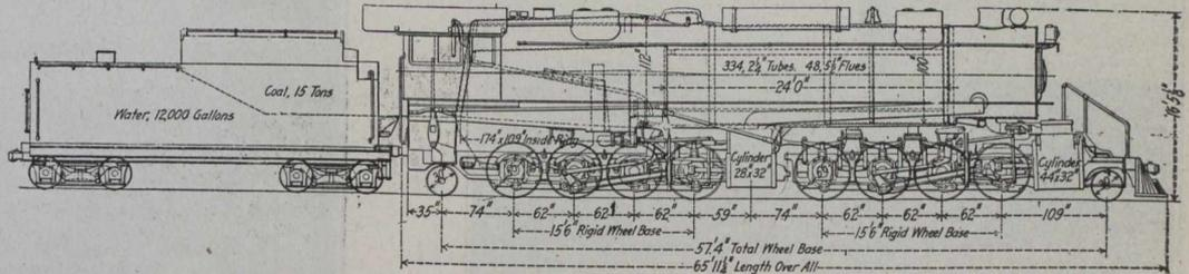
With two of these Mallets as helpers and a Mallet of 92,000 lbs. tractive power as a road engine, it is expected to take a train of 4,230 tons over a 14 mile, 2.07% grade. This grade is the ruling point on the entire line as all the tonnage passes over it. The road engine will then take the train unaided through to the terminal of the division.
