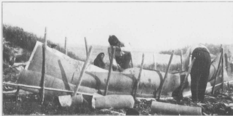
SAULTEAUX CANOE-MAKING: Placing upper barks in position and trimming.
