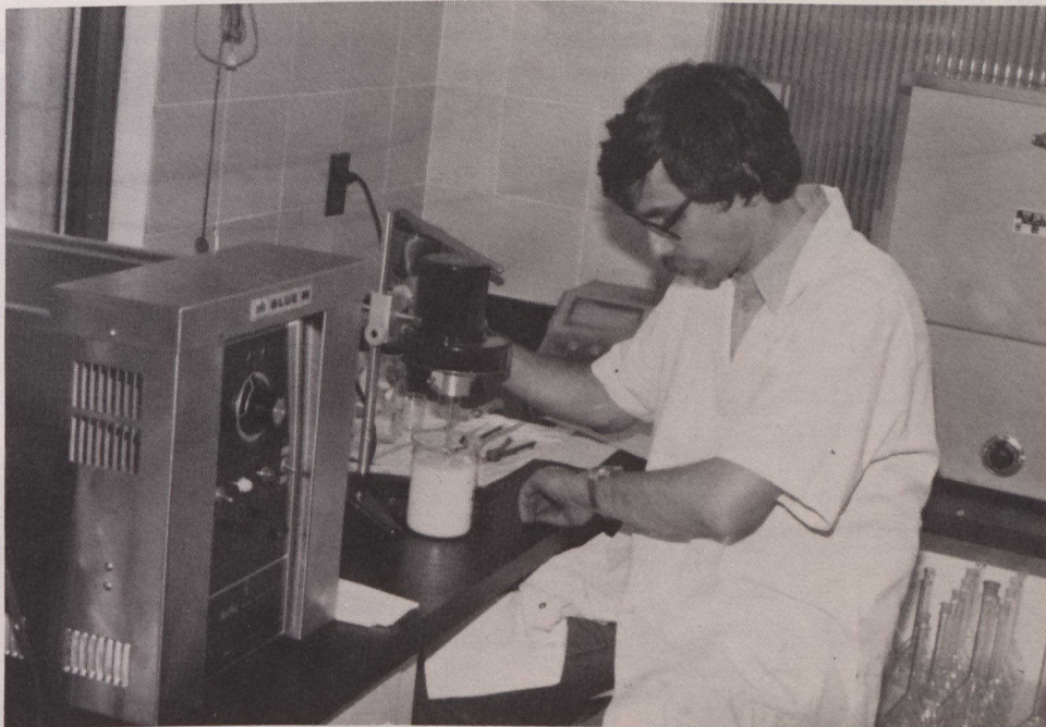
Development of a fortified skim milk sterilized by the ultra high temperature system with added milk proteins and vitamins, has been completed. Dairy employee Lester Dobosz measures the viscosity of the finished product.
