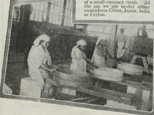
C OO-LIE girls at work in Lipton's factory in Ceylon. They shake the huge sieves which separate the tea leaves from pebbles, twigs and other foreign matter. Green and black tea are picked from the same plant. The preparation constitutes the difference in colour.
