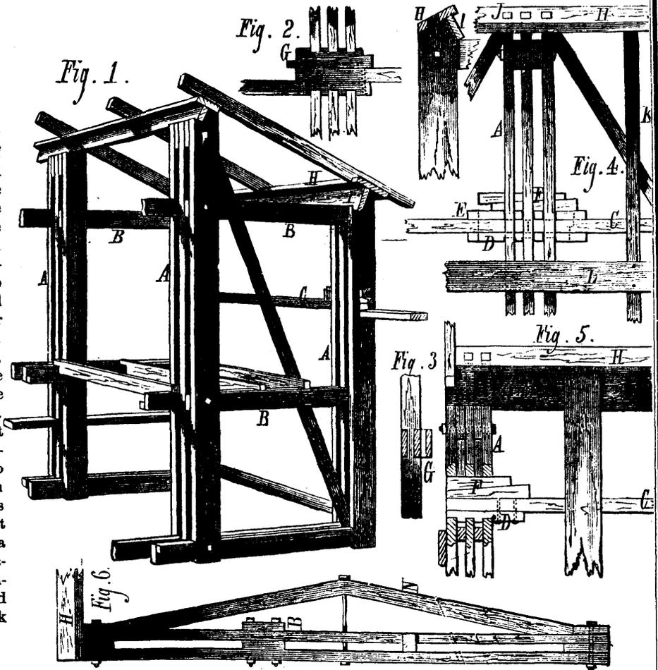
posts, and are rigidly secured at their meeting ends by a recessed key D, Figs. 4 and 5, which is first passed through the mortises of the post and then placed in position. The girder ends, after being inserted, are connected with a second recessed top key, E, of less width. Both keys are spiked to the girder ends in order to unite them. The keys and girder joints are finally locked to the mortises of the plank post by two wedge keys, F, introduced at relatively opposite directions.
