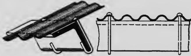
Fig. 25. Clinch Nail Fastening for Corrugated Iron Roofing.
