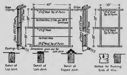
Fig. 44. Monitor Roof Skylight of Translucent Fabric.
