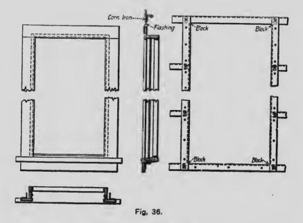
Figs. 34 to 36. Details for Side Window in Brick and Iron Frame Walls.
