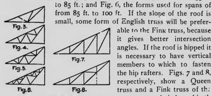
Figs. 3 to 8. Diagrams of Common Forins of Roof Trusses.
