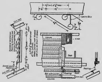
Fig. 38. Monitor Roof Ventilator with Louvres.
