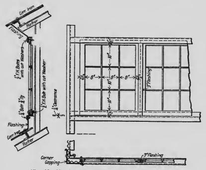
Fig. 40. Montior Roof Ventilator with Fixed Sash.
