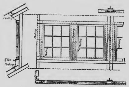
Fig. 41. Monitor Roof Ventilator with Movable Sash.
