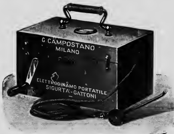
FIG. 97.—DR. SIGURTA'S PORTABLE DYNAMO FOR ELECTRIC LIGHT.
