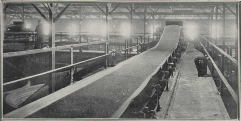
UPPER STORY OF A GRAIN STOREHOUSE—THE GRAIN TRAVELS ON A RUBBER BELT AT THE RATE OF 700 FEET PER MINUTE ON ITS WAY FROM THE WEIGHING BIN TO THE STORAGE TANKS. A SIMILAR ARRANGEMENT TAKES IT FROM THE BOTTOM OF THE TANKS BACK TO THE ELEVATOR FOR LOADING ON CARS OR SHIPS.
