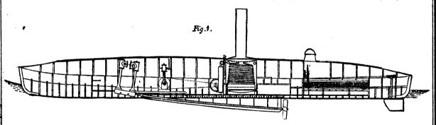
Fig. 2.—MACHINERY OF HERRESHOFF TORPEDO LAUNCH.
