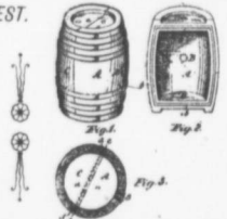
FIG. 1 Is an exterior view of the Cask. FIG. 2 Is an interior perspective view of one section of the Cask. FIG. 3 Is a transverse horizontal section through middle of Cask.
