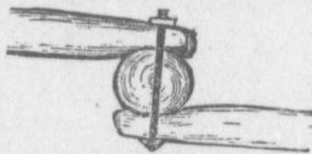
Fig. 33.—MODE OF SECURING RAILS.
