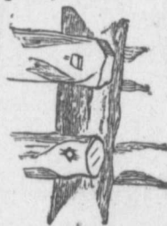
Fig. 34.—RAILS SECURED TO POSTS.
