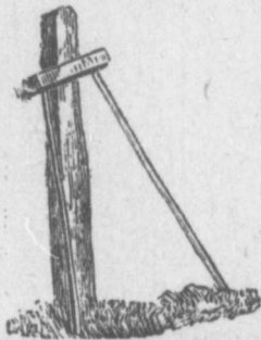
Fig. 15.—TWO LEGGED HORSE FOR SUPPORTING RAILS—LEANING AGAINST POSTS.
