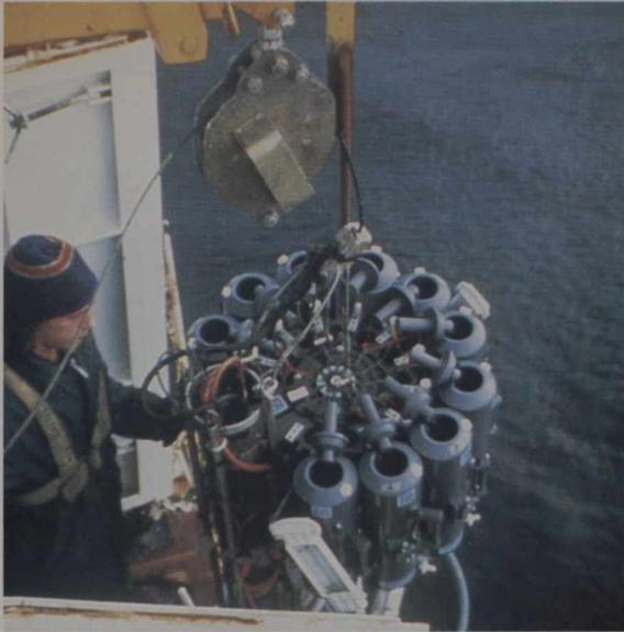
*An instrument cluster used for water sampling.*
