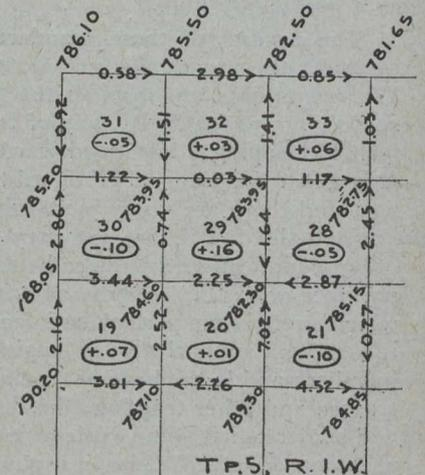
**Specimen Diagram Showing Closures in Each Square Mile (Eliminated by Adjustment)**
