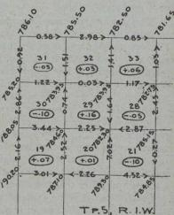
Specimen Diagram Showing **Closures in Each Square Mile** (Eliminated by Adjustment)
