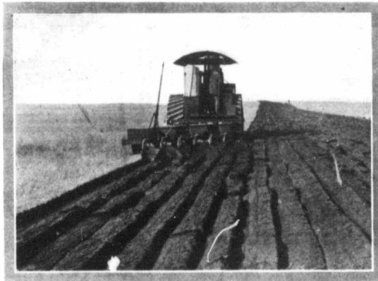
A Hart Parr 45 H.P. Gas Tractor negotiating some heavy sod with a 6 bottom John Deere Engine Gang. At work near Kindersley, Sask.
