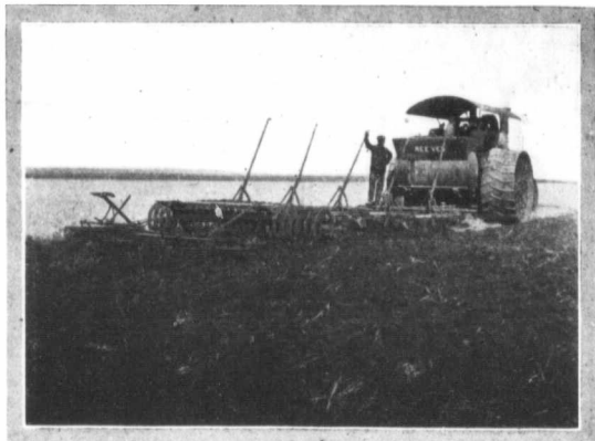
A Reeves Steam Tractor Pulling a 10-Bottom John Deere Engine Gang with Packer and Drag Harrow, near Swift Current, Alta.
