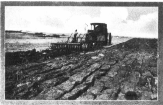
Avery Undermounted Steam Tractor pulling an 8 bottom Cockshutt Engine Gang and a Soil Packer near Cardston, Alta.
