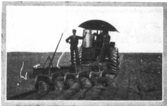
A Hart-Parr 45 h.p. Kerosene Tractor Pulling 6 14-inch John Deere Bottoms, at Castor, Alta.
