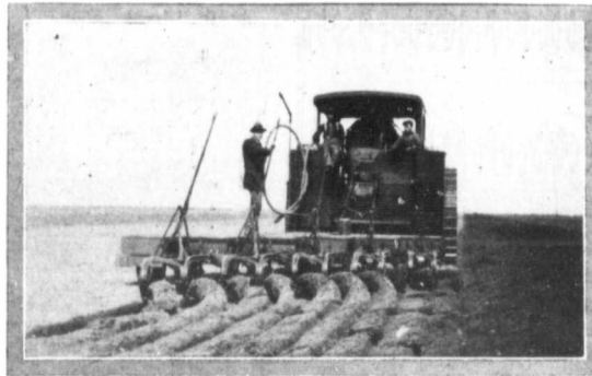
An Avery Undermounted Steam Tractor pulling a 10-bottom 14-inch John Deere Engine Gang, near Cardston, Alta.
