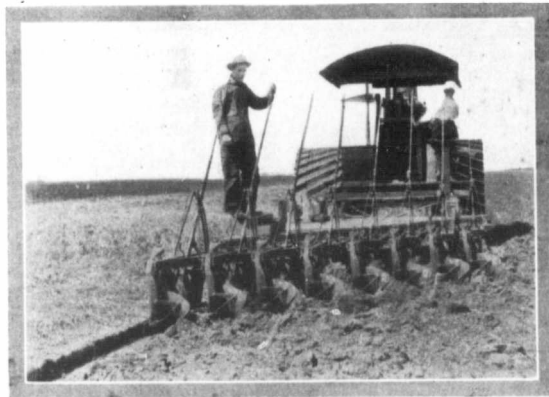
A Big Dutchman Engine Gang and a Hart-Parr 45 h.p. Gas Tractor at Work Near Portage la Prairie, Manitoba
