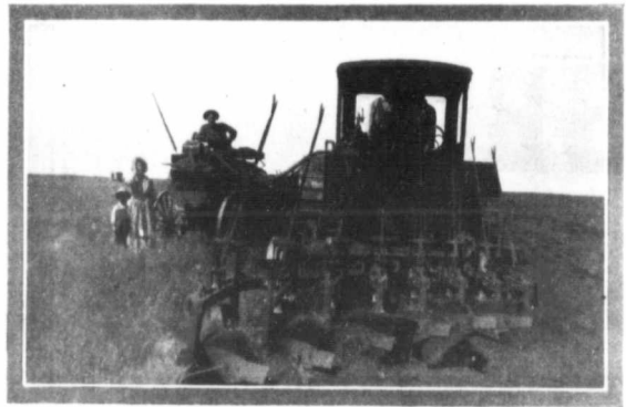
An Avery Undermounted Steam Tractor pulling an 8 bottom 14 in. Cockshutt Engine Gang.
