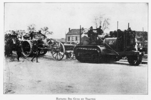
Thousands of these caterpillar tractors, made in the United States, were used in France to transport heavy guns to the front-line positions.
