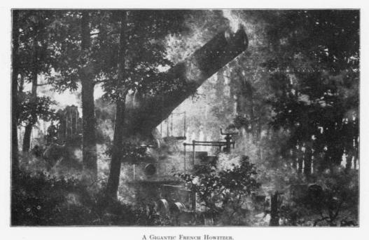
One of the mammoth guns built by France to batter the German positions. It is mounted on a specially built railway car and may be readily moved from one firing position to another.
