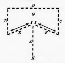
All the nets, A, B, C, D, E and F, are placed perpendicularly in the water, the foot being sunk to the bottom by means of lead, and the head supported on the surface by floats, represented on the diagram by the thick lines. The space G is occupied by a net which forms the bottom of the trap and is always sunk. Net A is called the leader, and, as is shown in the diagram, extends from the body of the trap to the land,
