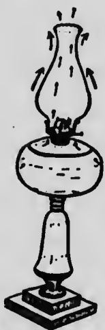
FIGURE 2.—Air moving upwards from a lighted lamp.
