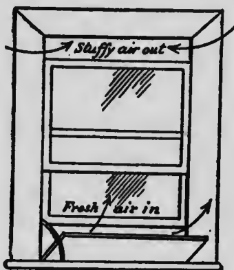
FIGURE 3.—Slanting board, arranged so that it can be adjusted to deflect the incoming draft upward. The upper sash lowered, the lower sash raised.
