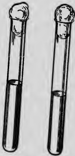
FIGURE 9.—Two test-tubes containing infusions that have been "sterilized" by boiling.
