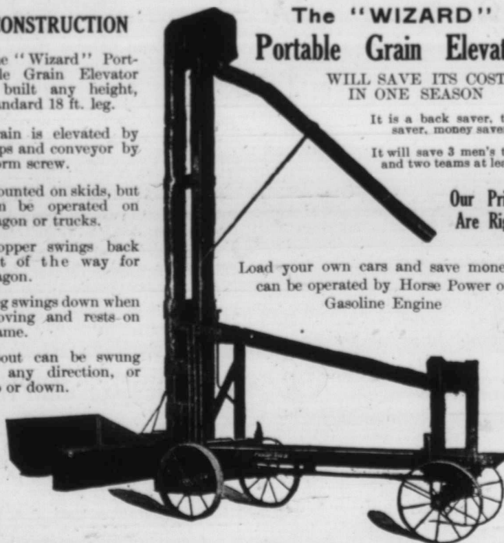
This cut shows Elevator mounted on truck, with leg up and hopper ready to receive grain. Write for prices and terms.
