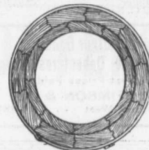
End view of Pipe and Coupling
