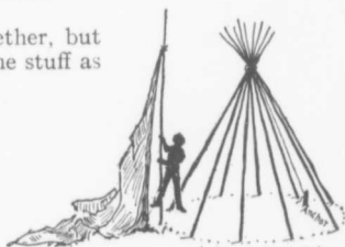
3 rd Set up tenth pole with teepee cover fastened to it by lash ropes.
