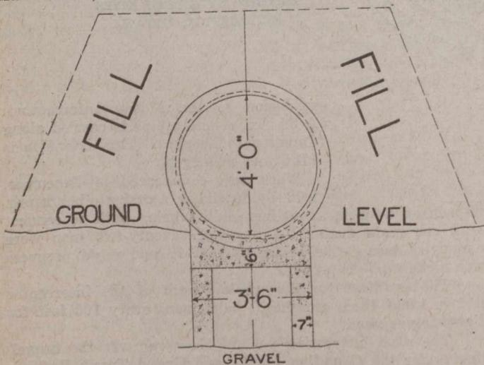
FIG. 3—METHOD OF SUPPORTING PIPE UNDER FILL
