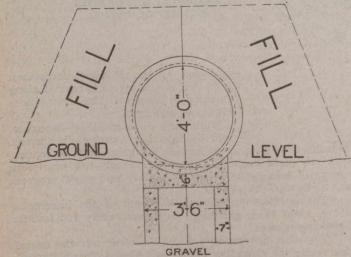
FIG. 3-METHOD OF SUPPORTING PIPE UNDER FILL
