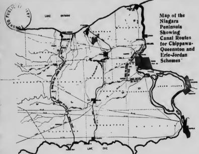
to adopt for the Hydro Power Canal, the route shown on the accompanying map. This route is about 1234 miles long, with the intake on the Niagara River at Hog Island, Chippawa, about two miles above Niagara Falls, and the tailrace on the Niagara River about one mile above Queenston. The intake will be in what is known as the Grass Island Pool of the Niagara River. The mean monthly elevation of this pool varies about 1 foot.
