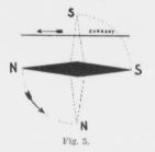
rent carrying wire wound around a frame with an indicating needle, which rotates around a fixed magnate. (See Fig. 3, p. 136).
