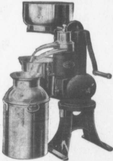
Note the heavy, compact construction and convenient height of supply can discharge spouts. The top of the supply can is only 3 1-2 ft. from the floor.
