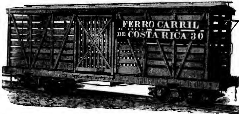
Length of frame,  $23\frac{1}{3}$  feet. Width, 7 feet. Wheels, 20 inches in diameter, fitted on  $3\frac{1}{8}$  inch axles with steeled iron trucks, and steeled spiral bearing springs encased.
