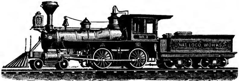
This engine has four connected drivers and a four-wheeled truck.
