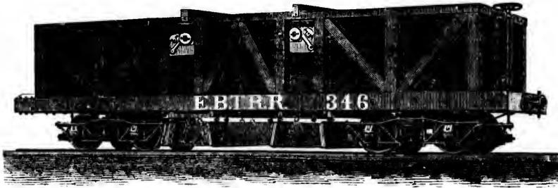
Length of frame,  $23\frac{1}{2}$  feet. Width, 6 feet. Wheels, 20 inches in diameter, fitted on  $3\frac{1}{8}$  inch axles with steeled iron trucks, and steeled spiral bearing springs encased.
