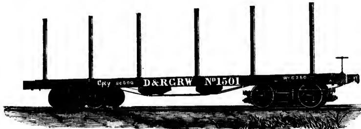
Length of frame  $23\frac{1}{2}$  feet. Width, 6 feet. Wheels 20 inches in diameter, fitted on  $3\frac{1}{8}$  inch axles with steeled iron trucks, and steeled spiral bearing springs encased.
