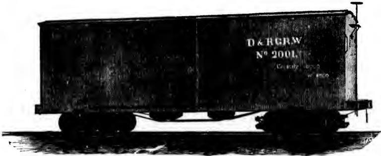
Length of frame,  $23\frac{1}{2}$  feet. Width, 6 feet. Wheels, 20 inches in diameter, fitted on  $3\frac{1}{8}$  inch axles, with steeled iron trucks, and steeled spiral bearing springs encased.
