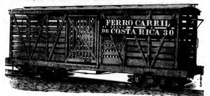
Length of frame,  $23\frac{1}{3}$  feet. Width, 7 feet. Wheels, 20 inches in diameter, fitted on  $3\frac{1}{8}$  inch axles with steeled iron trucks, and steeled spiral bearing springs encased.
