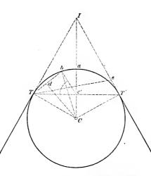
The random line T e is first run, and the angle I found by measuring I e T and I T e, and taking their sum from 180°. Then I T T' determined, and the chord T T' located. On this middle point, c' is taken as the station. Then if we lay off any line c' b, making an angle I with the chord, the distance on this line to the circle will be
