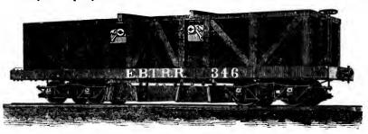
Length of frame,  $23\frac{1}{2}$  feet. Width, 6 feet. Wheels, 20 inches in diameter, fitted on  $3\frac{1}{8}$  inch axles with steeled iron trucks, and steeled spiral bearing springs encased.
