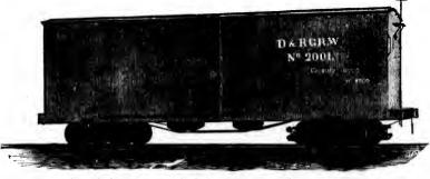
Length of frame,  $23\frac{1}{2}$  feet. Width, 6 feet. Wheels, 20 inches in diameter, fitted on  $3\frac{1}{8}$  inch axles, with steeled iron trucks, and steeled spiral bearing springs encased.
