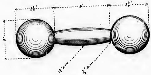
Next, find the centre of each of the larger parts, and mark it around with a pencil, and, using these centre lines as the starting-places for cuts, turn each end to the spherical form shown in Fig. 97, operating in the same manner that the convex curves were made in the regular third exercise. Turn the inside first and then the outside, cutting the ball a small amount inside the outer corner, that the spherical
