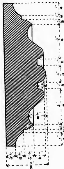
to the form shown in Fig. 81. This is done with the skew chisel, except the recess that is  $\frac{1}{8}$  inch in width, and this
