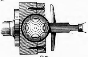
Over the wooden chuck used in turning the ball fit a wooden disk, and turn a hole in the centre of it, so that it may be fastened to the chuck with screws, and have a portion of the ball project through the
