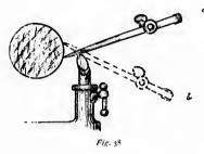
shown by the solid lines in Fig. 38. If held in the position shown by the dotted lines, they may catch into the wood
