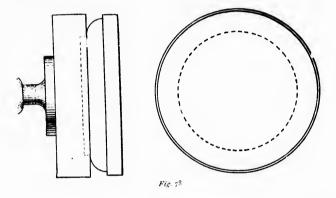
Next mark on the face of the outer disk a circle 4 inches in diameter and another 3 inch in diameter, and cut a recess 4 inch in depth between these marks with the skew
