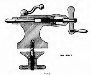
when it is desired to change it, by turning the *handle* until its back end strikes against the front end of the *screw*.
