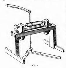
by the use of rude and imperfect tools. Some beautiful specimens of turned work have been made on the somewhat primitive tool shown in Fig. 1. This rude lathe, on which the work is revolved between two pointed metal pins held in two blocks of wood, contains the essen-
