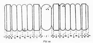
It will be found better to first cut grooves at the points of division, as shown in Fig. 45, as this helps to define the beads and keeps the size more nearly right. These grooves are cut in the same manner that the recesses in the second exercise were cut—with the acute corner of the chisel, the obtuse corner being held clear of the surface being cut. Use the obtuse corner in cutting the convex curves. Place
