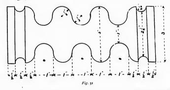
Turn the wood to a smooth cylinder 3 inches in diameter, and mark it to the dimensions shown in Fig. 53. Both concave and convex curves are to be half-circles in out-
