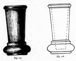
same manner that similar operations were performed during the regular eleventh exercise. The inside may be bored and then turned with the round-nose chisel, or the work may be done wholly with the skew-chisel. The skew-chisel may be used to finish the square corners.
