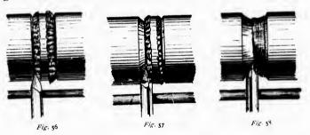
in Fig. 58, until it arrives at the position shown in Fig. 59. The cut is again started on the right-hand side, but with the edge nearer the boundary-line for the hollow, and the bevel more nearly a right angle with the axis of the work,
