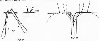
The aim should be to so combine the features shown that the cut will be a smooth and continuous one.
