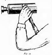
may be used as a guide in regulating the depth of the cut as the cutting edge is advanced to the end of the wood. Start the cut about 2 inches from the tail-stock end and produce it to the oth-
