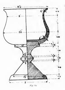
Prepare a chuck by attaching a piece of pine wood, four or five inches in diameter and one inch thick, to a face-plate, and turning it round and smooth; after which, with the face-plate still attached, remove it from the lathe and fasten to it the disk from which the bowl of the cup is to be made. This may be done by inserting a screw from the back through the opening for the lathe-spindle, as shown in Fig. 88.
