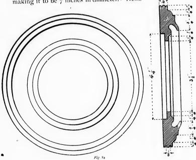
turn a recess in the face 44 inches in diameter and 4 inch in depth, and when this is done remove it from the face-plate. Put on instead of the disk just turned a pine one
