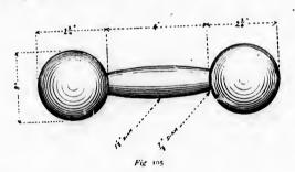
Next, find the centre of each of the larger parts, and mark it around with a pencil, and, using these centre lines as the starting-places for cuts, turn each end to the spherical form shown in Fig. 97, operating in the same manner that the convex curves were made in the regular third exercise. Turn the inside first and then the outside, cutting the ball a small amount inside the outer corner, that the spherical
