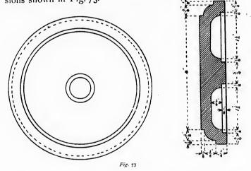
Fasten the disk to a face-plate with \(^3\_4\)-inch screws, placing the centre of the plate over the centre of the disk, and selecting such a face-plate that the holes left in the disk by the screws will be cut away in the subsequent turning—that is, the holes made by the screws must come in some place where a recess will be turned in the disk. Screw the face-plate easily on the spindle of the head-
