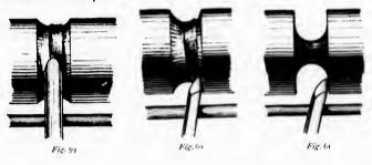
Next cut the convex portion of the curve by placing the gouge in the position shown in Fig. 62, and using it
