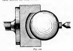
Prepare a chuck of the form shown in Fig. 102, and fit it to the ball, as shown. The ball may be held in place by putting a small piece of thick leather against
