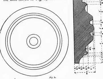
to the torm shown in Fig. 81. This is done with the skew chisel, except the recess that is k inch in width, and this
