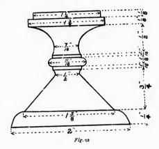
Put the second piece of stock between the lathe-centres, and turn from it the stem to the form and dimensions shown in Fig. 92. Varnish and polish it before taking it from the lathe.
