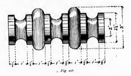
Turn a plain cylinder 3 inches in diameter, mark on it the lines that determine the convex curves, and reduce the remainder of the stock to a diameter of  $2\frac{1}{2}$  inches, and then cut the convex curves. Next, mark the position of the concave curves and cut them in the same manner that the concave curves were cut in the regular fourth exercise.
