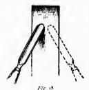
as before, by drawing the edge through a piece of wood, or it may be "buffed" off by rubbing the edge on a leather strap or on the palm of the left hand.
