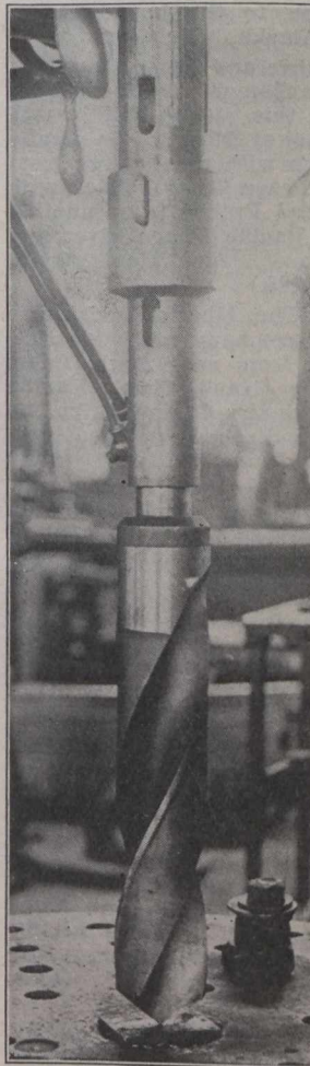
Socket to Hold Larger Drills than Spindle Socket Allows For.
