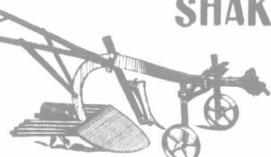
Natural temper steel blade. Weed Fender and gauge wheel. The Shaker Digger has a perfectly flat blade and will not cut the potatoes. The back grating shakes the earth clear and leaves the potatoes clean and on top of the ground.
