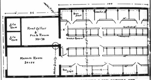
GROUND PLAN - BASEMENT BARN OF H. CARGILL & SON, CARGILL, ONT. Size of Basement Walls 72 x 156 feet. Concrete floors put in this building with Thorold Cement.
