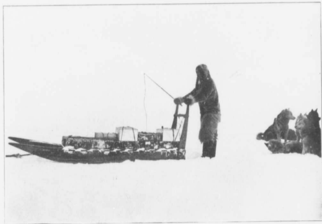
ESKIMO TYPE OF SLEDGE USED ON JOURNEY 9 ft. 6 in. Long, 2 ft. Wide, 8 in. High; With Steel Shoes 1½ in. Wide Each has standard load of supplies for team and driver for fifty days— pemmican, biscuit, milk, tea, oil, alcohol
