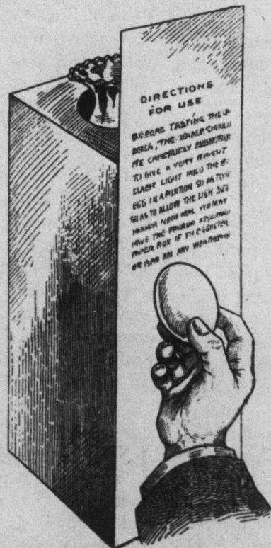
A paste-board egg-candling device given free to merchants by Agricultural Department, Dominion Government, for distribution among farmers.
